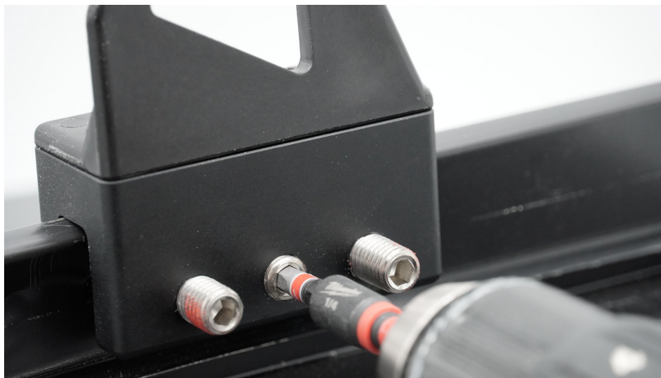
Figure 2 — Driving the set screws. A 5 mm hex bit on an extension keeps the bit square to the screw, which prevents cam-out and uneven seating.
