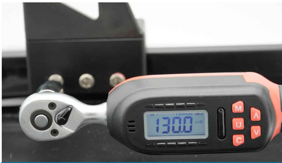
Figure 3 — Final torque. Confirmed at 130.0 in-lb. A wrench that reads in inch-pounds is required — a standard foot-pound wrench does not resolve this range accurately.
