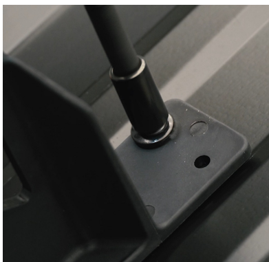
Figure 3 — Driving the fasteners. An 8 mm socket on a driver set to a clutch setting, not impact mode.
